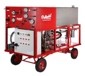
When high flow rates at high pressures are needed, the booster can charge a receiver to an even higher pressure level, storing a volume of gas available for rapid release at a constant pressure through a pressure reducing valve.
