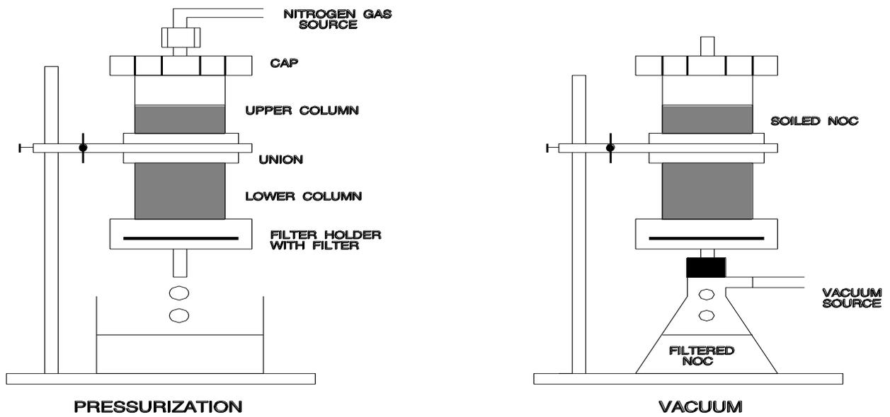
FIGURE 3. Filtration for determining NVR in NOC by gravimetric.
