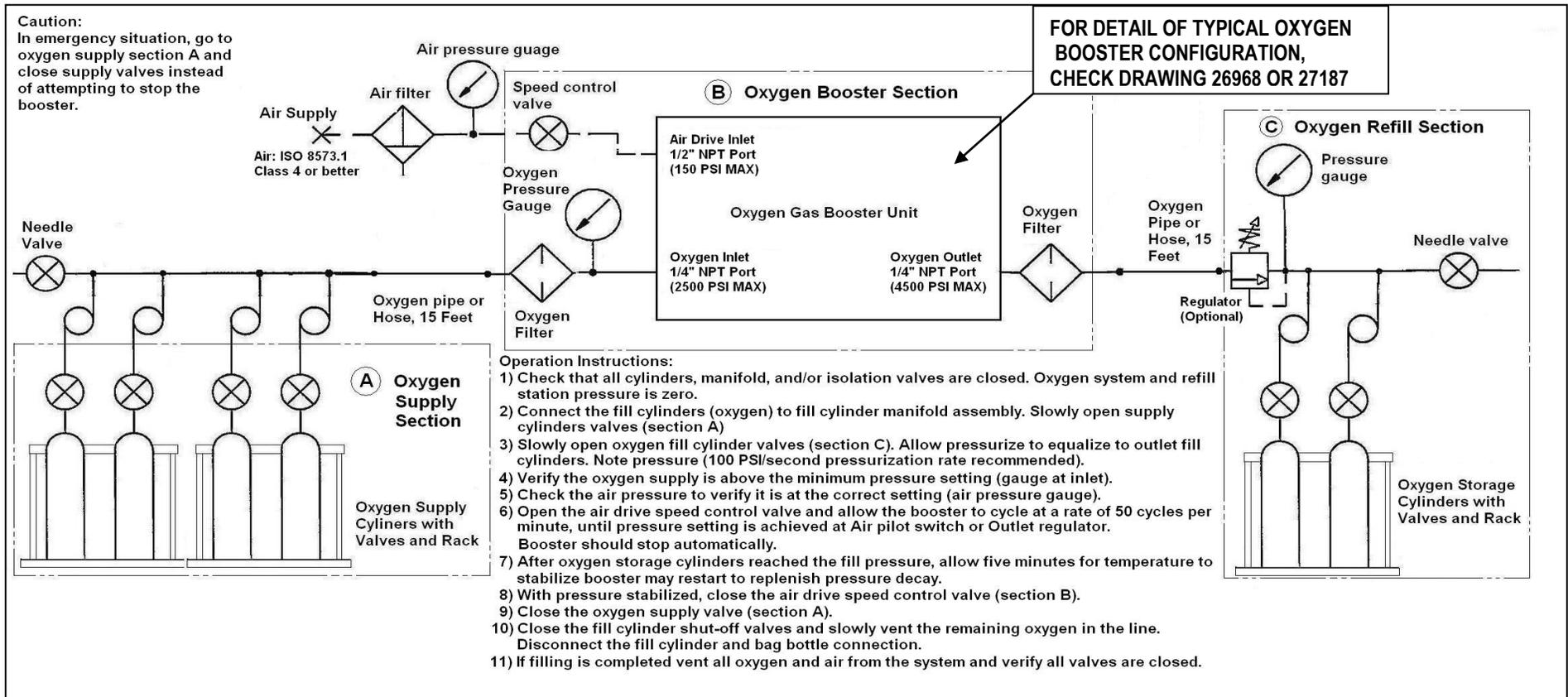
**Fig. 2 -Typical Configuration of Haskel Oxygen System and Operation Instructions**
